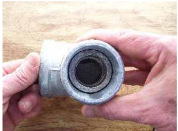
The holder fits in this end to hold the fitting tightly and sealing for the resin pour.
