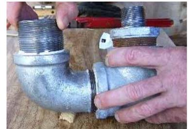
Here you can see how this unit fits into the other fittings to form the base. Left, the unit screws into the 2" tee. Middle, the bushing for the clack valve screws into the top of the 2" tee. Right, the 2" close nip screws into the top of the check mount unit.
