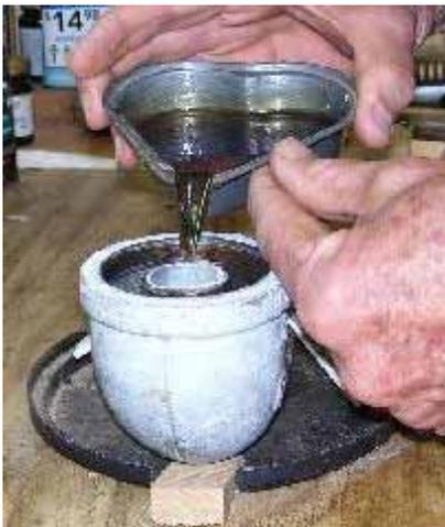
The second pouring will seal any small gaps that may have formed from the resin pulling away from the inside of the fitting. This rarely happens, generally only when the resin gets too hot. Bring the level up to the bottom thread of the 1" fitting. *We no longer rely on a gasket seal where the check valve seats on the resin. We rely on the tapered threads of the fittings to seal the check valve to the mount.*
