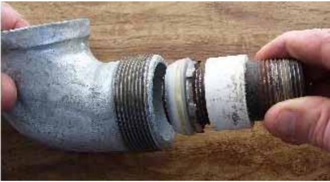
First insert the holder tool carefully into the 2" ell. It should be smooth inside and the fit firm but not too tight. Get the threads started into the 1" ell inside, do not tighten. *When tightened later* the putty will be squeezed out between the two plastic washers and should seal perfectly. The PVC collar on the holder tool should help center the tool as well. The inside of this fitting and the 2" close nip should be **ground** smooth.
