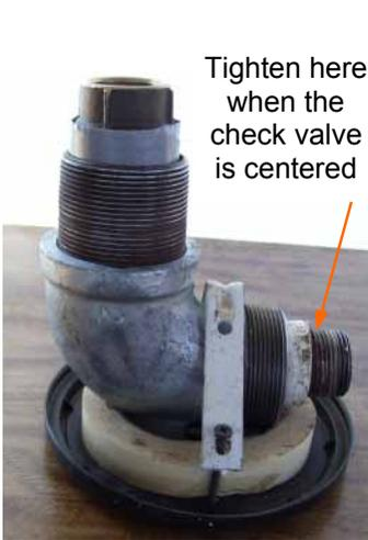
After centering the taped check valve, mount the whole unit to the bench -- I use a roll of masking tape and an angle iron. The purpose is to secure the thing in a level position.
