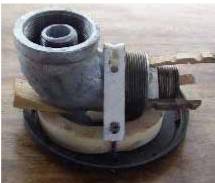
Here you can see the unit ready for the resin pour. Be sure to check the level and especially the centering again using a clean check valve and 2" close nip. Polyester resin (fiberglass) is to be mixed and poured into the gap between the fittings and filled to the first threads on the 2" fitting. Carefully lubricate the threads so no resin can stick to them.
