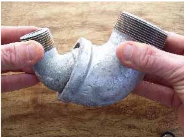
The 1" (smaller) fitting must fit loosely so it can be centered perfectly.
