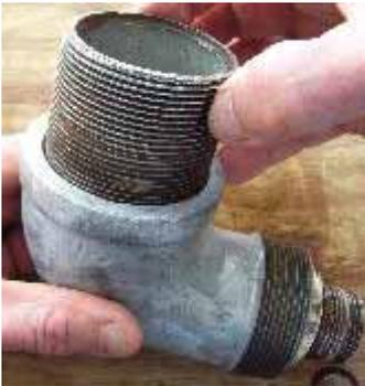
Next thread in the 2" close nip to the 2" ell (check mount). In order to center the check mount as perfectly as possible, use a check valve with a couple of wraps of duct tape around the body. Thread this valve into the 1" street ell inside the check mount. This should get the valve centered. This is tricky but necessary as the clearance is close and resin is unforgiving.
