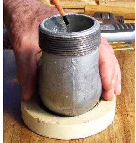
1" ell in the same way, from both sides. Watch those threads! When cured, a shot of gloss black spray paint inside the 2" and 1" ells will hide most any visible defect and help prevent the threads from rusting as well. Really only cosmetic. Below, note that the fitting may appear to be off center (left). You can test this with a check valve and the 2" close nip to be sure.
